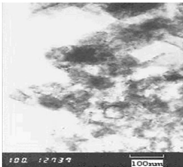
Figure 1 TEM micrograph of CaCO 3 nanoparticles.
